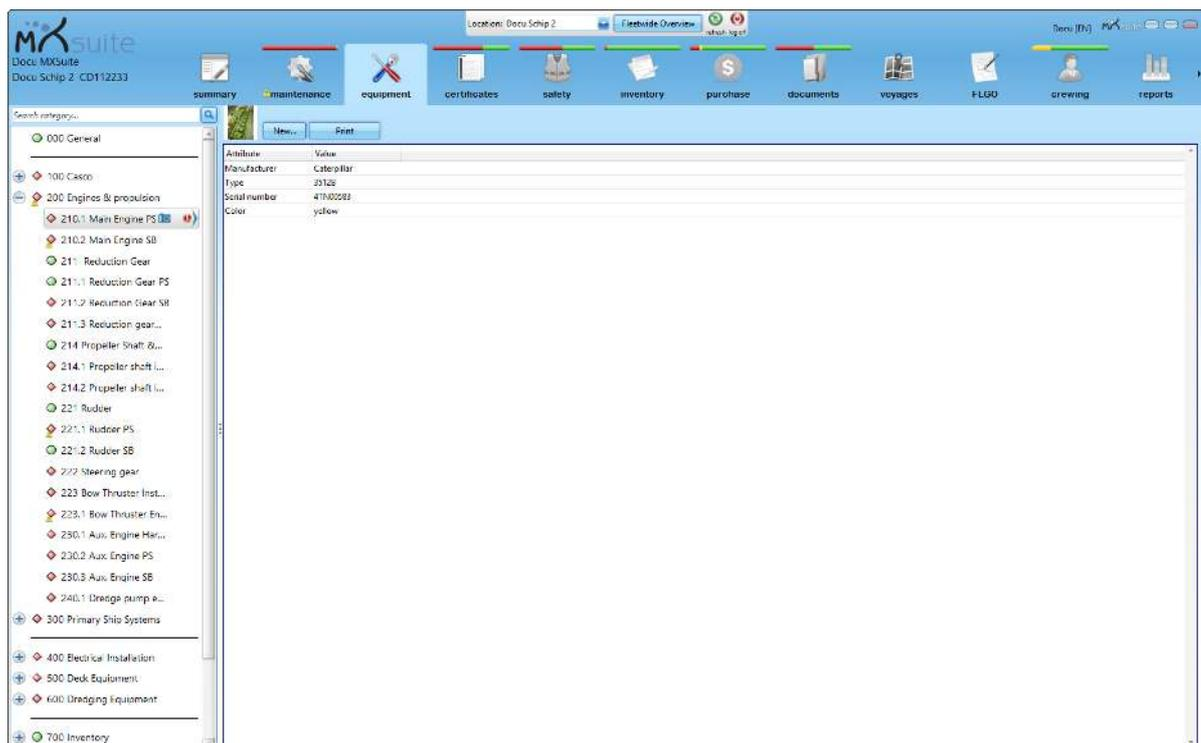
The module Equipment is used to save all data associated with the installed equipment such as the manufacturer, type, serial number, etc.
