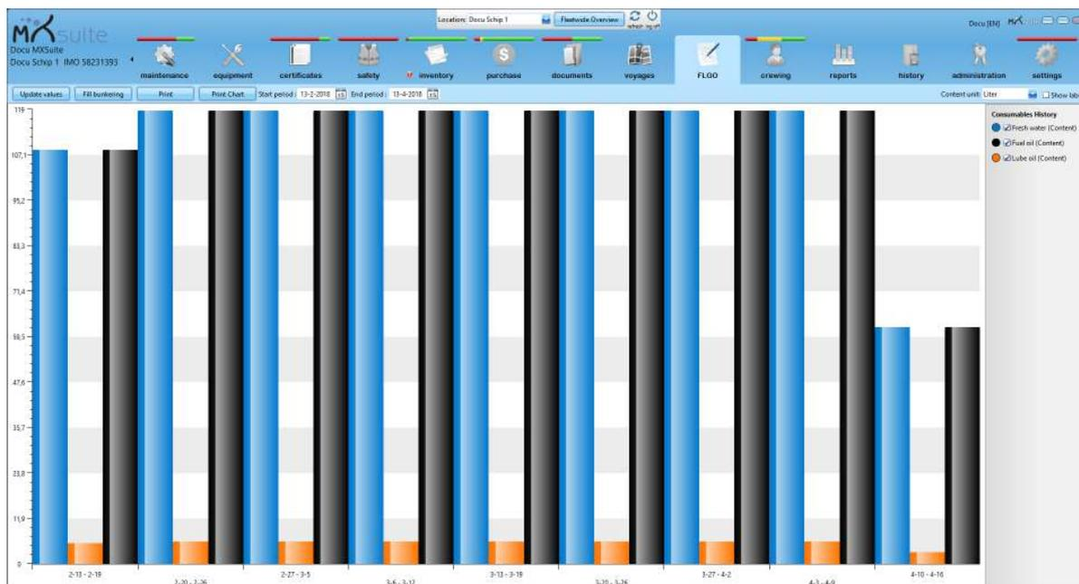
FLGO stands for **F**uel, **L**ube and **G**as **O**il. By regularly entering the actual stock and all bunkered quantities, the module FLGO can calculate the consumption of each preferred period. This provides insight into consumption and costs.
